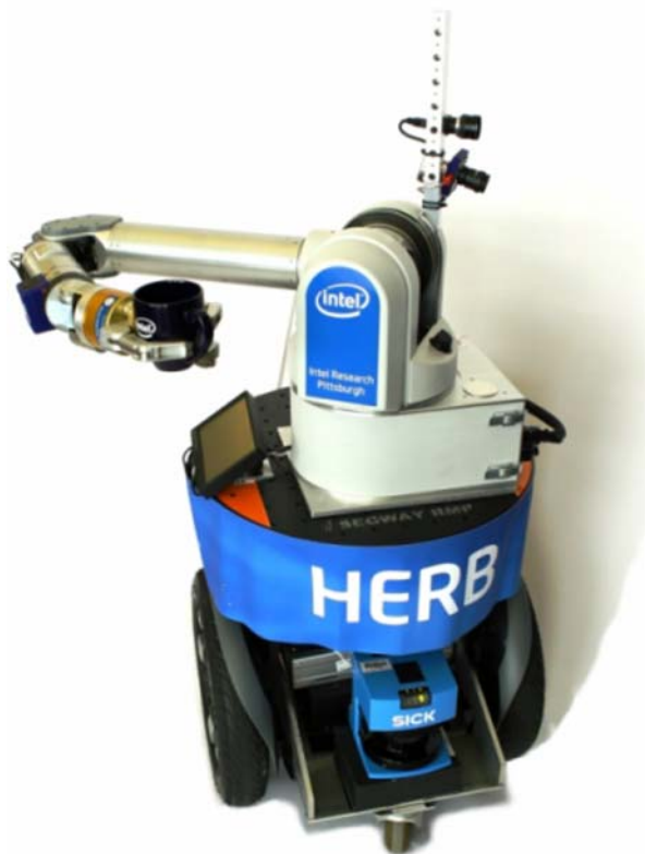
Fig. 1 Herb: a platform for Personal Robotics developed jointly by Intel Research Pittsburgh and Carnegie Mellon University
