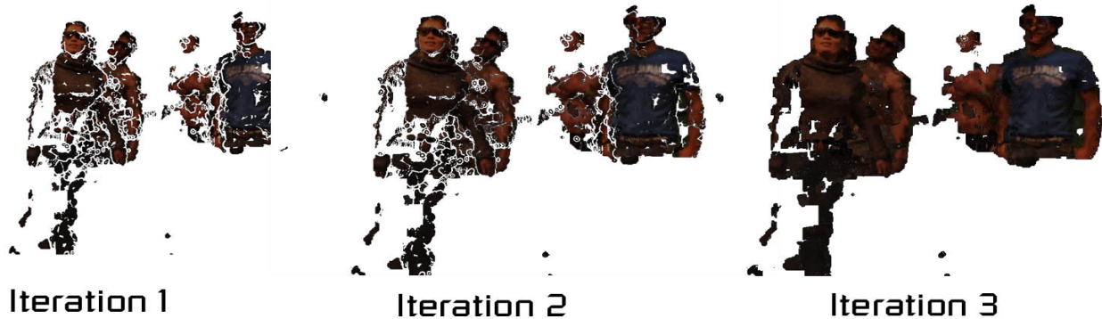
Figure 5: Adaptive Point Splatting performs multiple iterations over the point cloud. In each iteration, it relaxes the conditions for pixel rejection.
